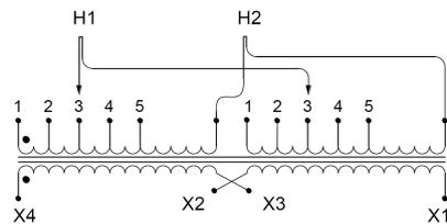
Single Phase Isolation Transformer with a capacity of 100kVA, transforming 575 Volts to 460 Volts
