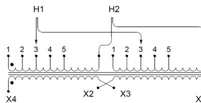
Single Phase Isolation Transformer with a capacity of 100kVA, transforming 240 Volts to 220/440 Volts
