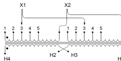
Single Phase Isolation Transformer with a capacity of 100kVA, transforming 220 Volts to 415 Volts
