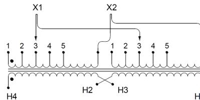
Single Phase Isolation Transformer with a capacity of 100kVA, transforming 120 Volts to 220/440 Volts
