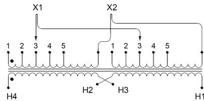
Single Phase Isolation Transformer with a capacity of 100kVA, transforming 115 Volts to 400 Volts
