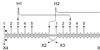
Single Phase Encapsulated Isolation Transformer with a capacity of 75kVA, transforming 575 Volts to 120/240 Volts
