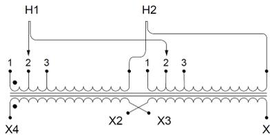
Single Phase Encapsulated Isolation Transformer with a capacity of 5kVA, transforming 600 Volts to 120/240 Volts
