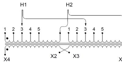
Single Phase Encapsulated Isolation Transformer with a capacity of 50kVA, transforming 600 Volts to 120/240 Volts
