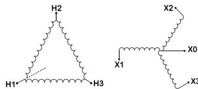
Three Phase Encapsulated Isolation Transformer with a capacity of 2kVA, transforming 480 Volts to 380Y/220 Volts
