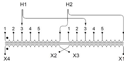
Single Phase Encapsulated Isolation Transformer with a capacity of 25kVA, transforming 460 Volts to 120/240 Volts
