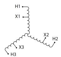
Three Phase Encapsulated Autotransformer with a capacity of 9kVA, transforming 480Y Volts to 208Y Volts
