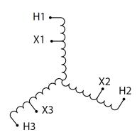
Three Phase Encapsulated Autotransformer with a capacity of 75kVA, transforming 600Y Volts to 480Y Volts
