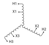
Three Phase Encapsulated Autotransformer with a capacity of 75kVA, transforming 600Y Volts to 240Y Volts
