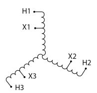
Three Phase Encapsulated Autotransformer with a capacity of 45kVA, transforming 600Y Volts to 208Y Volts
