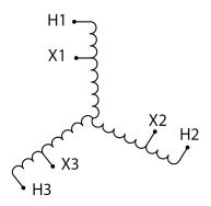
Three Phase Encapsulated Autotransformer with a capacity of 45kVA, transforming 480Y Volts to 208Y Volts
