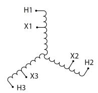
Three Phase Encapsulated Autotransformer with a capacity of 3kVA, transforming 600Y Volts to 208Y Volts
