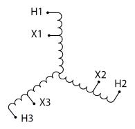
Three Phase Encapsulated Autotransformer with a capacity of 3kVA, transforming 480Y Volts to 240Y Volts
