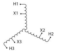
Three Phase Encapsulated Autotransformer with a capacity of 30kVA, transforming 600Y Volts to 480Y Volts
