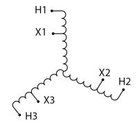
Three Phase Encapsulated Autotransformer with a capacity of 30kVA, transforming 600Y Volts to 208Y Volts
