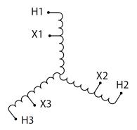
Three Phase Encapsulated Autotransformer with a capacity of 30kVA, transforming 600Y Volts to 208Y Volts
