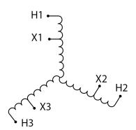
Three Phase Encapsulated Autotransformer with a capacity of 30kVA, transforming 480Y Volts to 240Y Volts
