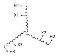
Three Phase Encapsulated Autotransformer with a capacity of 30kVA, transforming 480Y Volts to 240Y Volts
