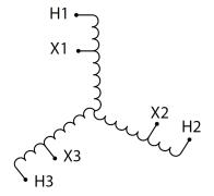
Three Phase Encapsulated Autotransformer with a capacity of 15kVA, transforming 600Y Volts to 480Y Volts
