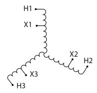
Three Phase Encapsulated Autotransformer with a capacity of 15kVA, transforming 600Y Volts to 240Y Volts
