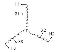
Three Phase Encapsulated Autotransformer with a capacity of 150kVA, transforming 600Y Volts to 480Y Volts
