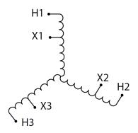
Three Phase Encapsulated Autotransformer with a capacity of 150kVA, transforming 600Y Volts to 480Y Volts
