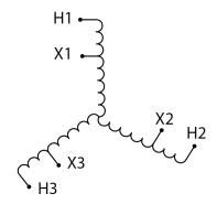
Three Phase Encapsulated Autotransformer with a capacity of 150kVA, transforming 480Y Volts to 208Y Volts
