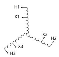
Three Phase Encapsulated Autotransformer with a capacity of 112.5kVA, transforming 600Y Volts to 480Y Volts
