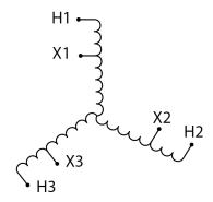
Three Phase Encapsulated Autotransformer with a capacity of 112.5kVA, transforming 480Y Volts to 208Y Volts
