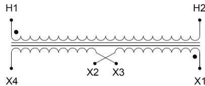
Single Phase Control Transformer with a capacity of 75VA, transforming 600 Volts to 120/240 Volts
