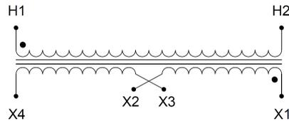
Single Phase Control Transformer with a capacity of 50VA, transforming 480 Volts to 240/480 Volts
