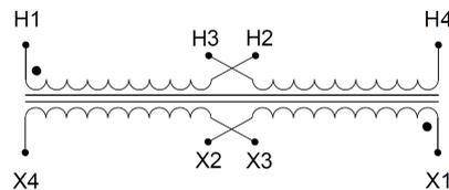
Single Phase Control Transformer with a capacity of 50VA, transforming 120/240 Volts to 240/480 Volts
