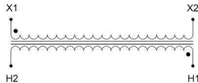
Single Phase Control Transformer with a capacity of 500VA, transforming 600 Volts to 120 Volts
