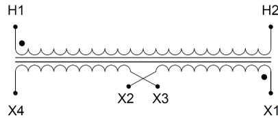
Single Phase Control Transformer with a capacity of 500VA, transforming 600 Volts to 12/24 Volts
