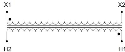
Single Phase Control Transformer with a capacity of 350VA, transforming 480 Volts to 120 Volts
