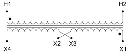
Single Phase Control Transformer with a capacity of 350VA, transforming 277 Volts to 120/240 Volts
