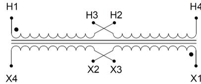
Single Phase Control Transformer with a capacity of 350VA, transforming 240/480 Volts to 12/24 Volts
