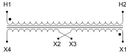
Single Phase Control Transformer with a capacity of 3000VA, transforming 600 Volts to 240/480 Volts
