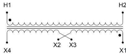
Single Phase Control Transformer with a capacity of 3000VA, transforming 277 Volts to 120/240 Volts
