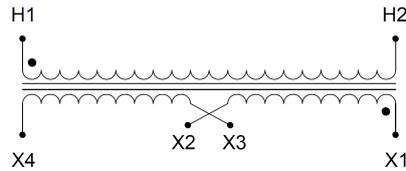
Single Phase Control Transformer with a capacity of 250VA, transforming 600 Volts to 120/240 Volts
