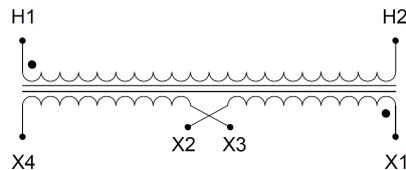
Single Phase Control Transformer with a capacity of 250VA, transforming 600 Volts to 12/24 Volts
