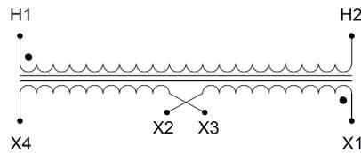
Single Phase Control Transformer with a capacity of 250VA, transforming 208 Volts to 120/240 Volts
