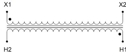
Single Phase Control Transformer with a capacity of 2000VA, transforming 600 Volts to 120 Volts
