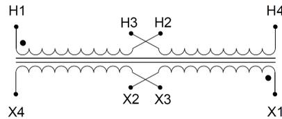
Single Phase Control Transformer with a capacity of 150VA, transforming 120/240 Volts to 12/24 Volts
