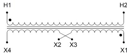
Single Phase Control Transformer with a capacity of 1500VA, transforming 600 Volts to 120/240 Volts
