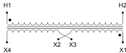
Single Phase Control Transformer with a capacity of 100VA, transforming 600 Volts to 120/240 Volts
