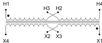
Single Phase Control Transformer with a capacity of 100VA, transforming 120/240 Volts to 12/24 Volts
