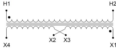
Single Phase Control Transformer with a capacity of 1000VA, transforming 480 Volts to 240/480 Volts
