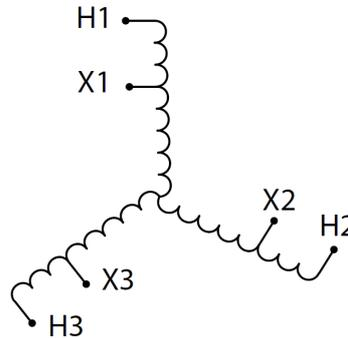
Three Phase Autotransformer with a capacity of 9kVA, transforming 600Y Volts to 110Y Volts
