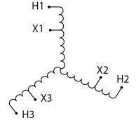
Three Phase Autotransformer with a capacity of 9kVA, transforming 600Y Volts to 110Y Volts
